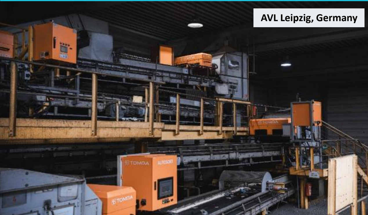
A modern packaging sorting plant can contain up to 60 NIR sorters
